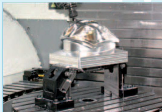
1246 - Machining on 5 sides with one single clamping operation
