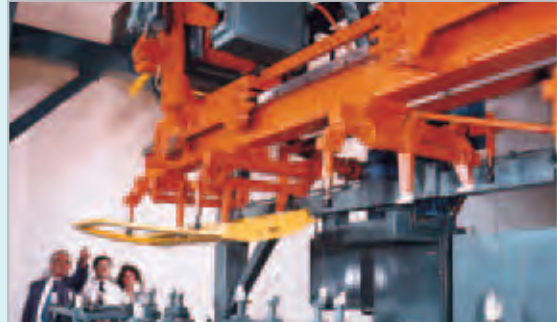
Bumpers are utilised to guide and align an automotive door in transfer machines for in-process assembly.
