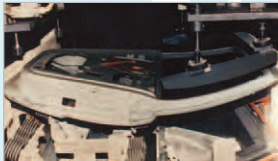
Rollers and bumpers guide and align an automotive door in bonding and curing applications.
